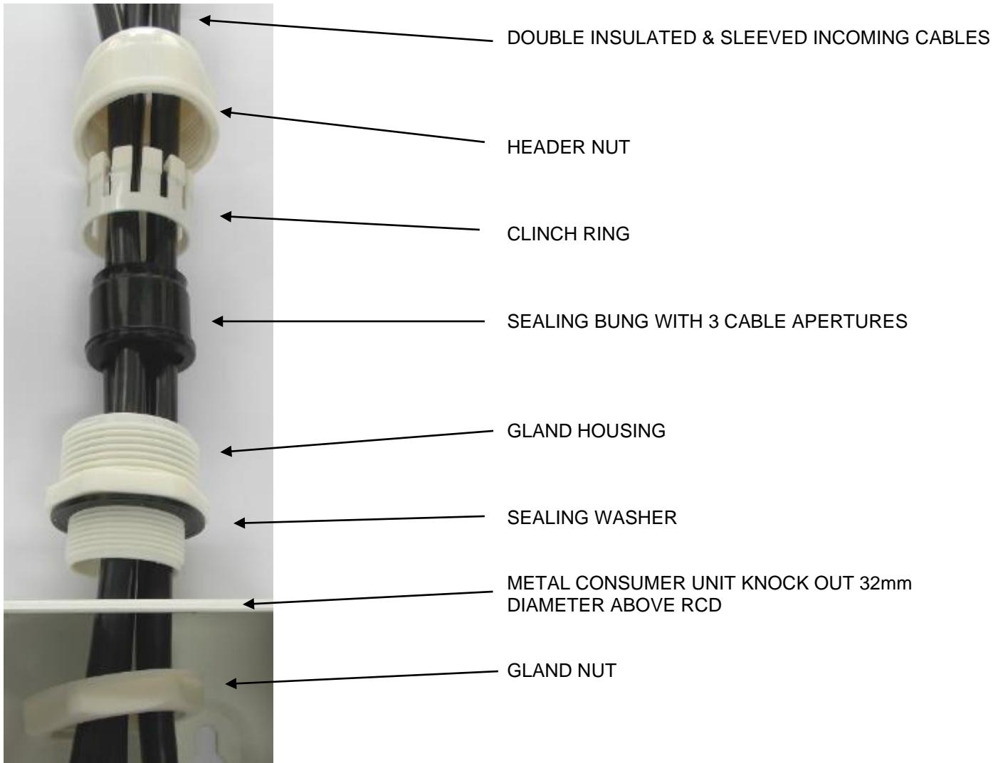
The kit comprises a 32mm insulated cable restraining gland, which is fitted by removing the knockout above the incoming terminals and fixing into position with the nut included. The incoming supply cables must be passed through the 3 aperture sealing bung.
